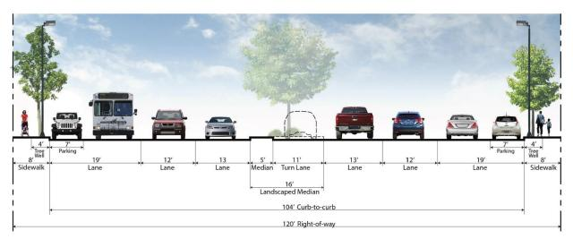
Figure 2 – Existing Typical Cross-Section
