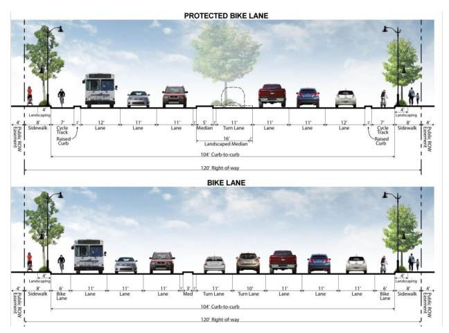
Figure 3 – Proposed Typical Cross-Sections
