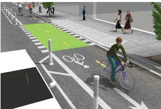
Example of bicycle lane buffer
