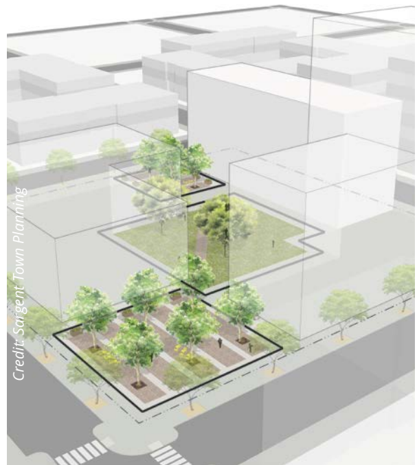
On-site open space should be visible from adjacent streets and/or buildings and at the same level as the public sidewalk
