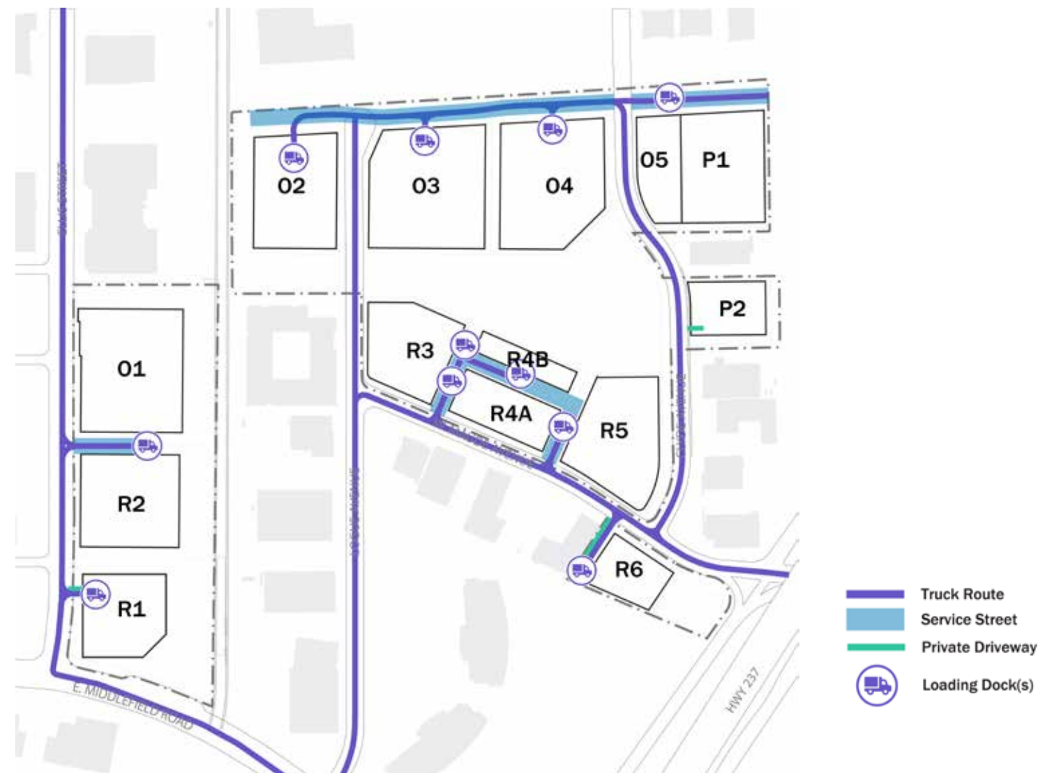
Figure 7.7.2 Truck access and routing
