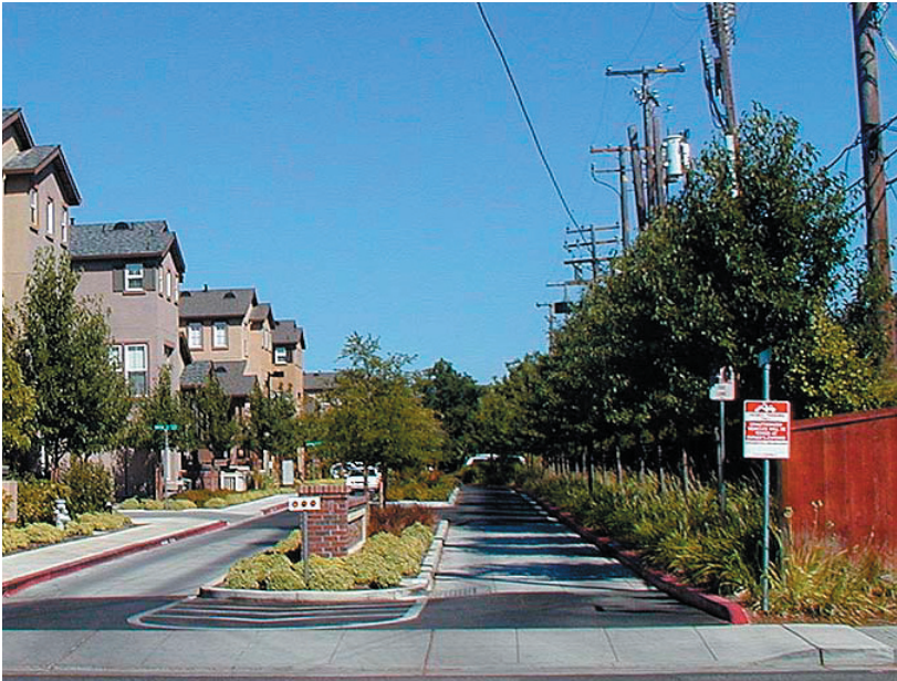
Internal streets should include a 5 foot minimum landscaped buffer when they run along property lines.
