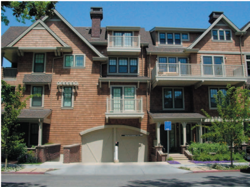
The number of structured parking entrances should be kept at a minimum and should be located on side streets or interior streets wherever possible.
