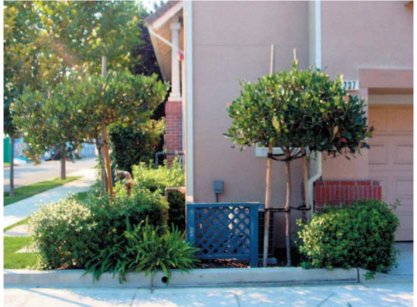
Utilities should be incorporated into the design of the building and integrated into landscaped areas to minimize noise and visual impact.
