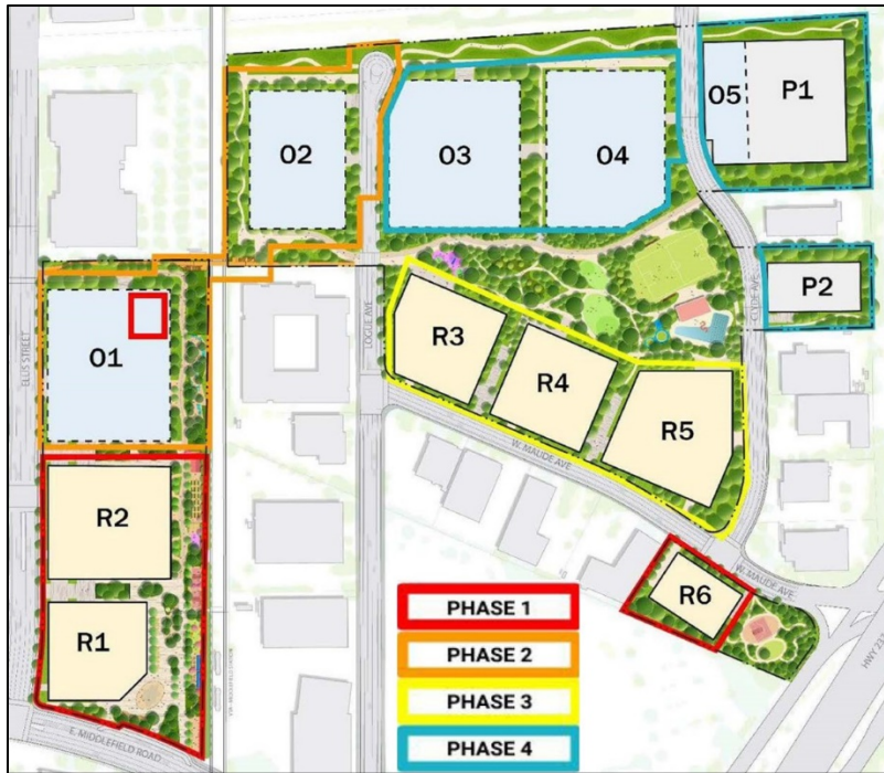
Figure 6: Conceptual Construction Phasing Plan
