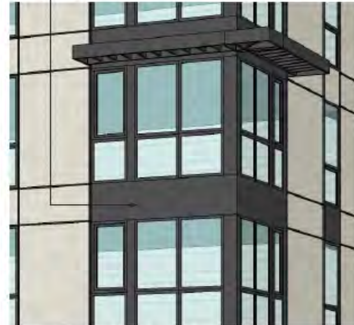
Hard-troweled acrylic-modified plaster
