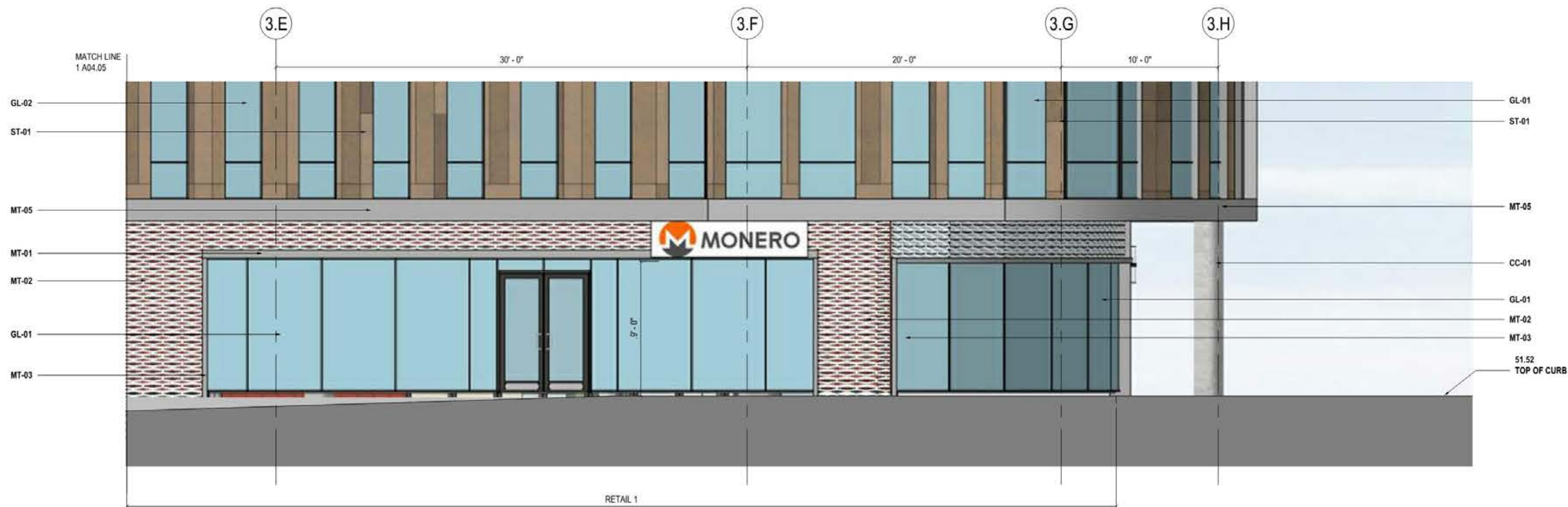
2 BUILDING ELEVATION - ENLARGED WEST (SOUTH SIDE) SCALE: 1/4" = 1'-0"
