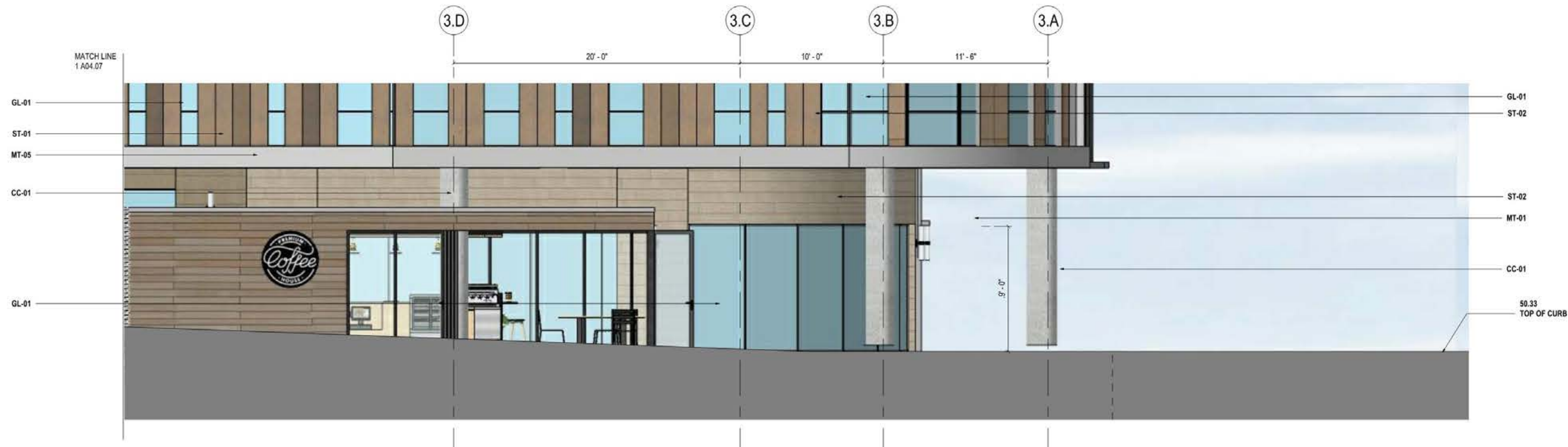
2 BUILDING ELEVATION - ENLARGED EAST (SOUTH SIDE) SCALE: 1/4" = 1'-0"
