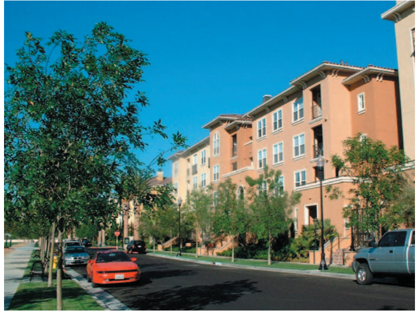
Internal Streets should conform to the high quality standards and be designed to resemble public streets, with sidewalks, parallel parking and street trees.
