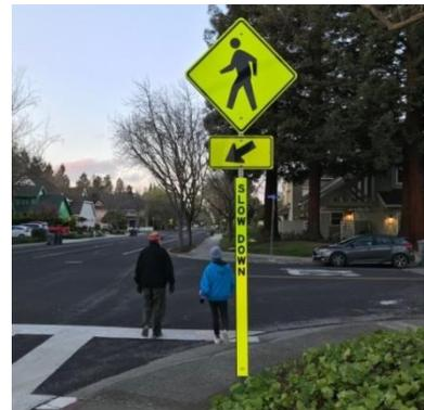
*Example of sign post panel reflector installed at an uncontrolled, marked crosswalk location on Sylvan Avenue*
