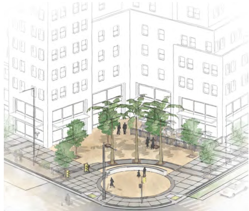
An example of a usable open area, configured as a public plaza situated at a corner. Building entrances are clearly visible and accessible from the sidewalk.
