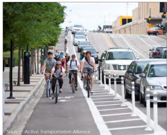
Class II bike facility with white buffer stripes and physical barrier.
