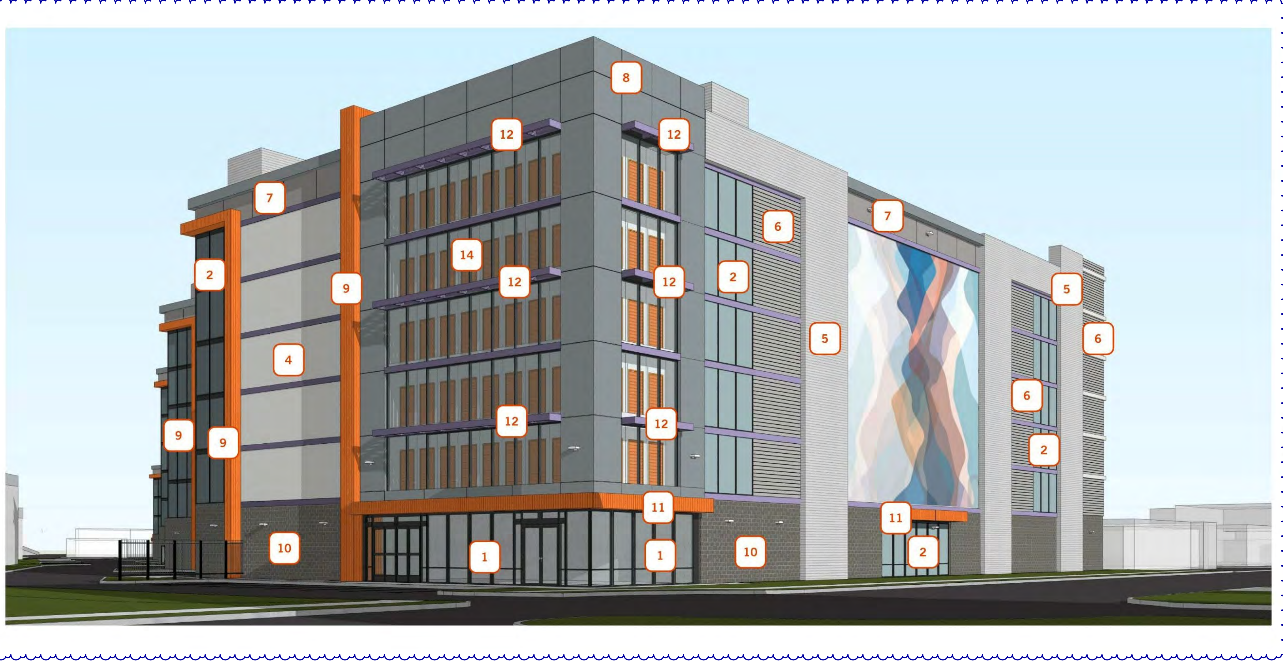
1 MULLIONS STOREFRONT: BLACK ANODIZED ALUMINUM MULLIONS WITH VISION GLAZING AND SLIDING DOORS AT ENTRIES
