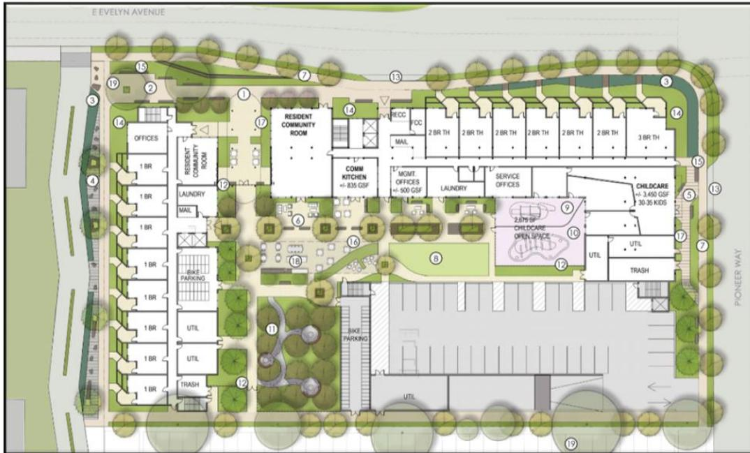
Figure 9: Alta Housing Proposal—Site Plan
