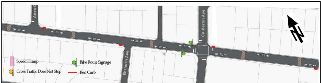
Figure 17 – Anza Street to Calderon Avenue Proposed Improvements
