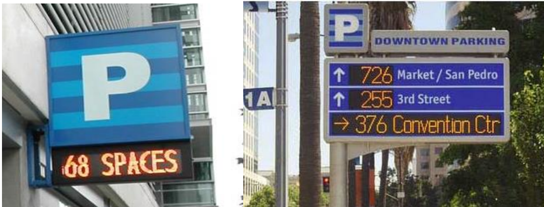
Figure 1-4: City of San Jose’s Dynamic Signage (entrance occupancy sign and directional sign)
