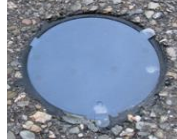
Figure 1-5: Embedded Parking Sensor
