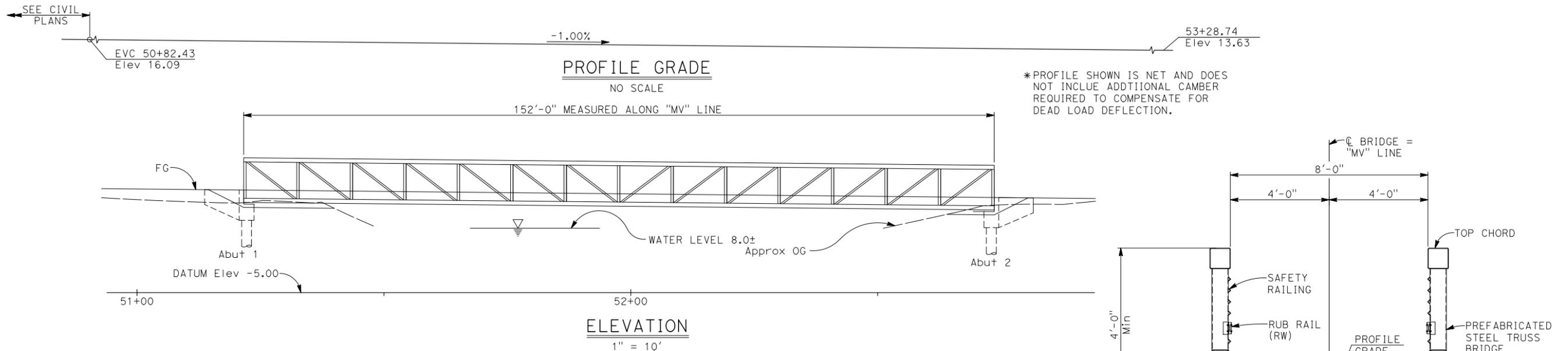
\*PROFILE SHOWN IS NET AND DOES NOT INCLUDE ADDITIONAL CAMBER REQUIRED TO COMPENSATE FOR DEAD LOAD DEFLECTION.
