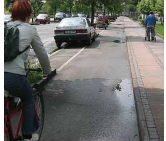
Buffered bike lanes like this one could be provided along California Street east of Pacchetti Way.
