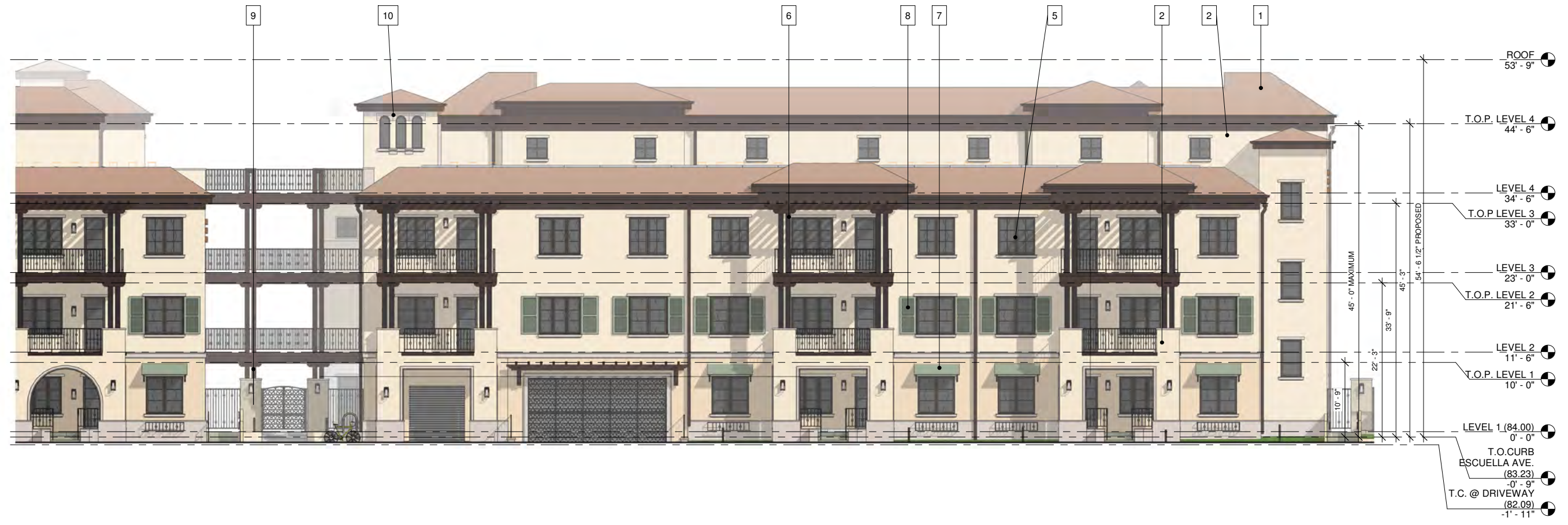
BUILDING B NORTH ELEVATION 1/8" = 1'-0" 1
