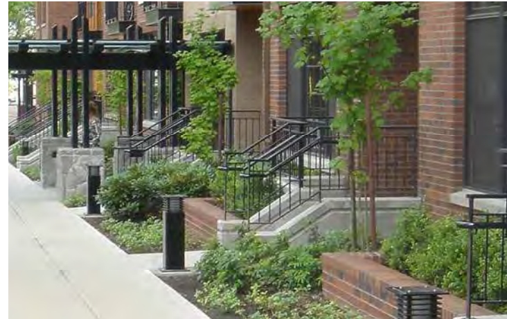
7l. Convey façade articulation through the strength, depth, and permanence of building materials. Thinner cladding materials, such as stucco, masonry veneers, and wood or simulated wood may be used when finished to appear as durable and authentic as the materials they simulate.
