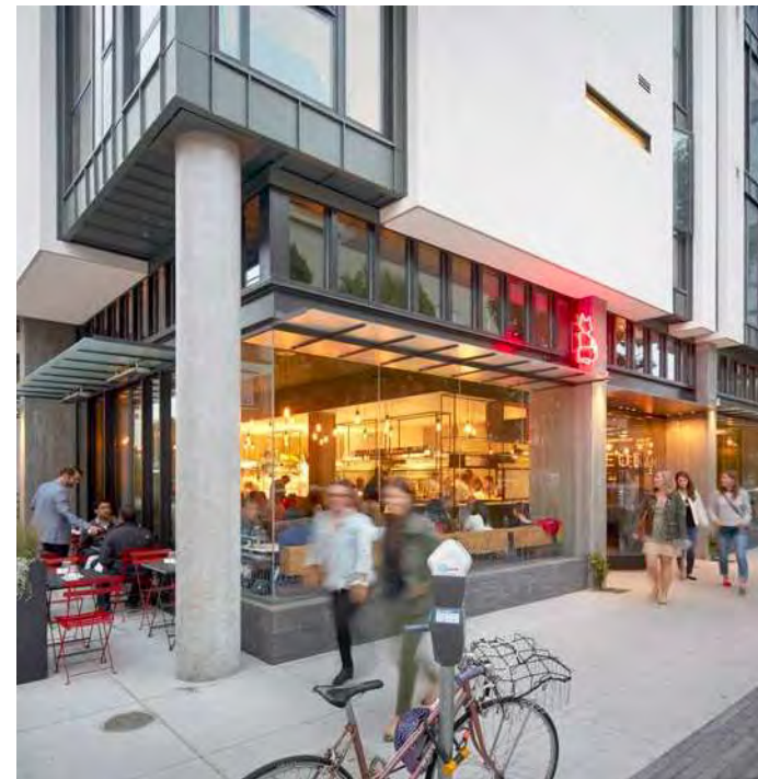
5c. Locate and orient active non-residential uses to public areas when ground floor dwelling units are not provided. Examples of active non-residential uses include community spaces, common areas, cafes, restaurants, retail, personal services, salons, gyms, grocery stores, banks, and pharmacies. Transparent retail shopfronts should be used in areas where active, pedestrian-oriented frontages are encouraged or required.
