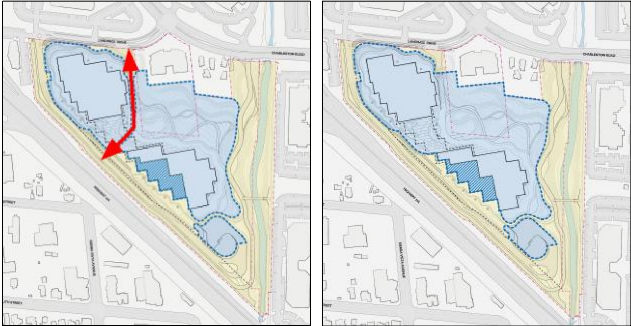
Left: North Bayshore Precise Plan's Conceptual Street through Site Right: Current Design without Vehicular Access through Site
