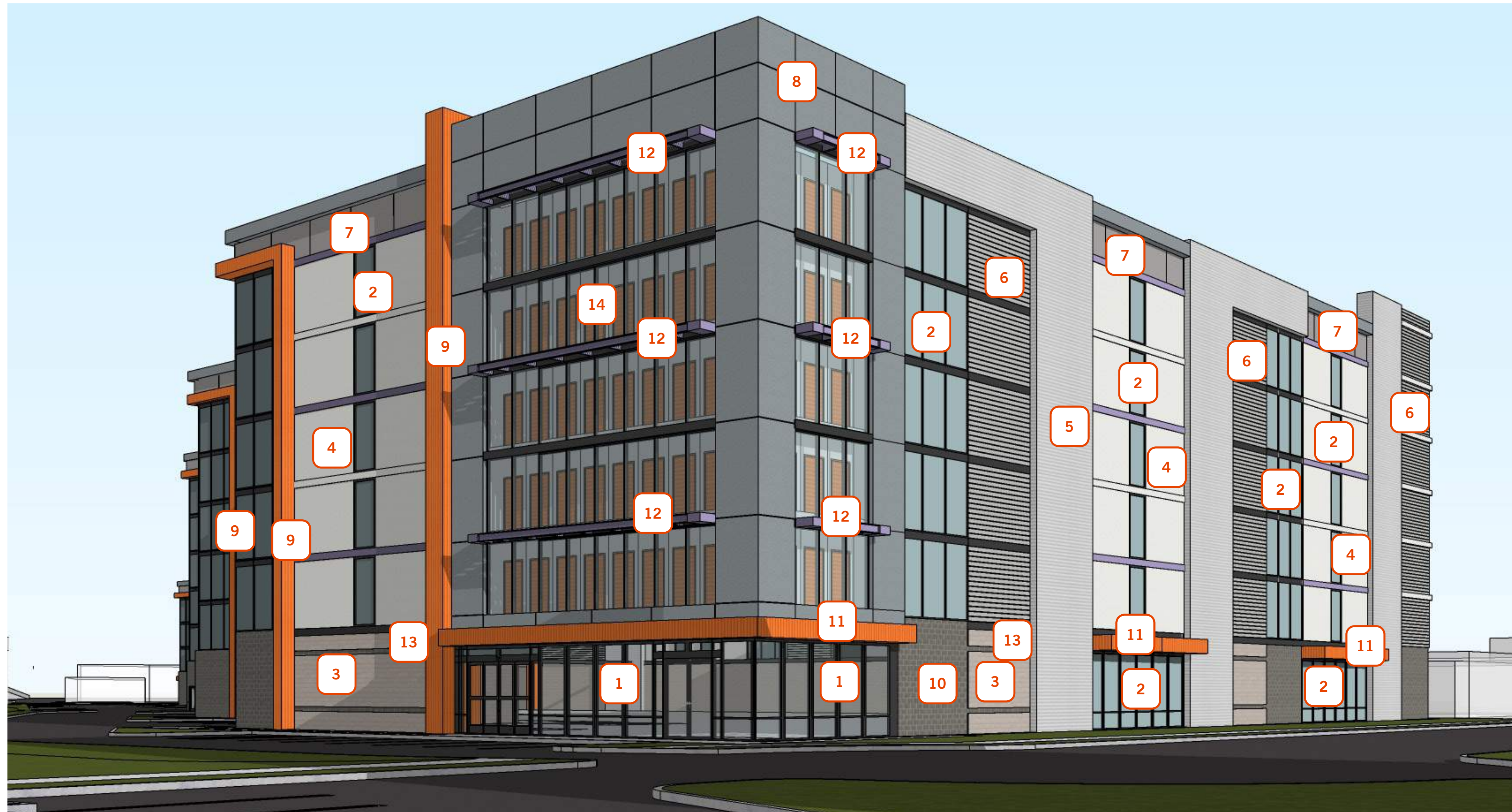
1 MULLIONS STOREFRONT: BLACK ANODIZED ALUMINUM MULLIONS WITH VISION GLAZING AND SLIDING DOORS AT ENTRIES
