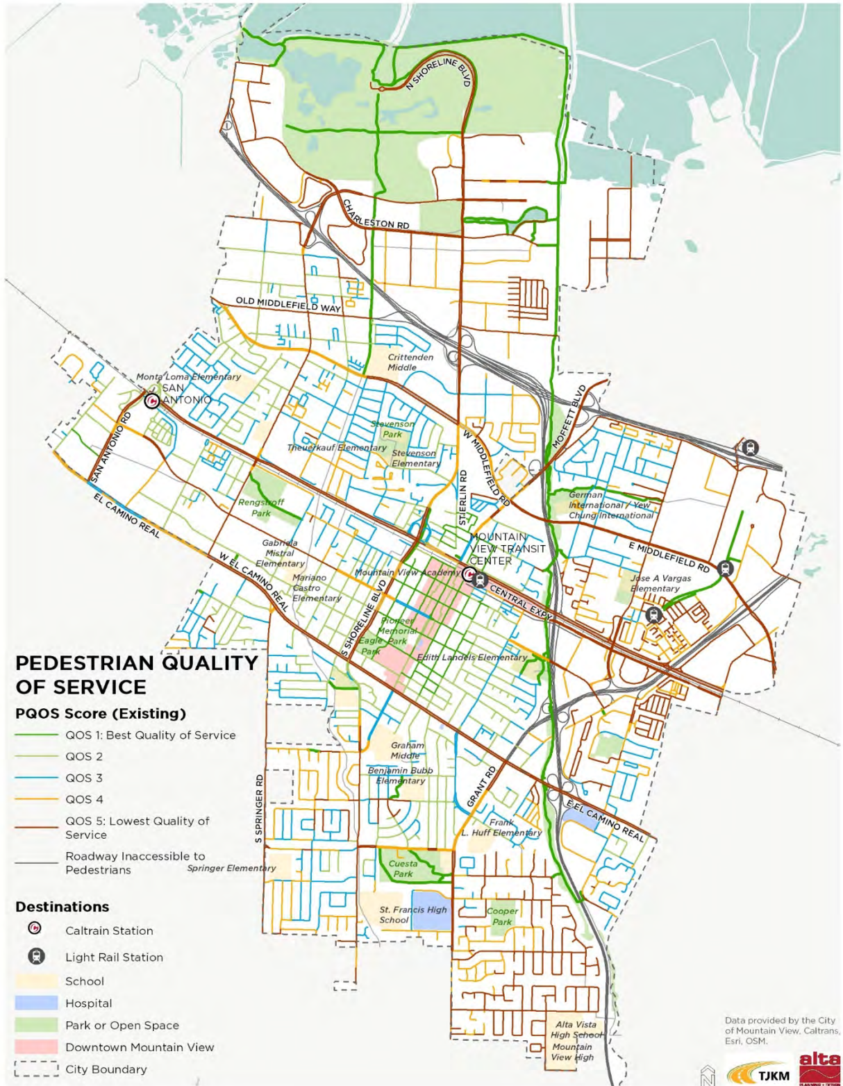
Figure 1. Pedestrian Quality of Service (Existing)
