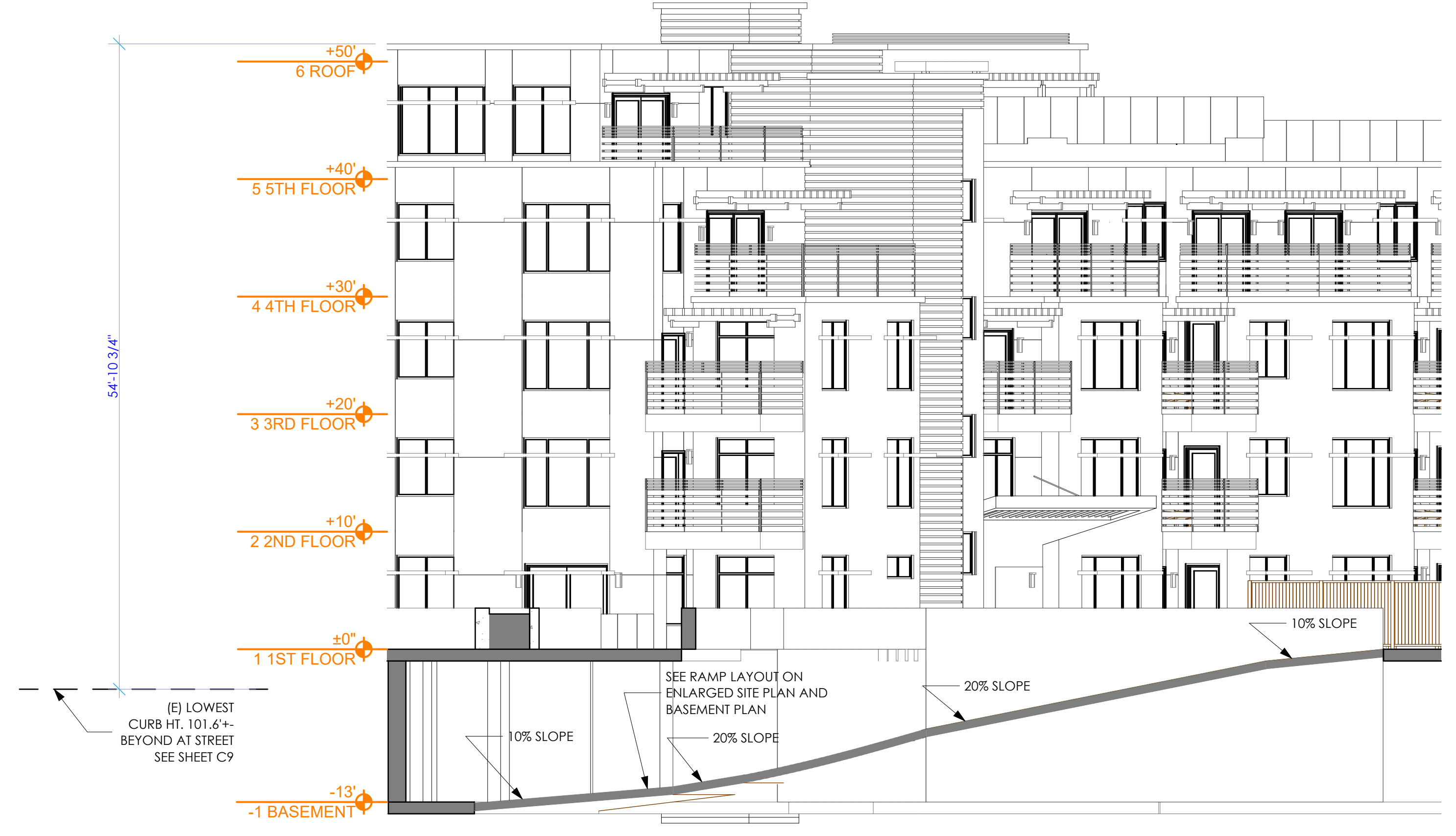
3 SECTION AT PARKING GARAGE RAMP SCALE: 1/8" = 1'-0"
