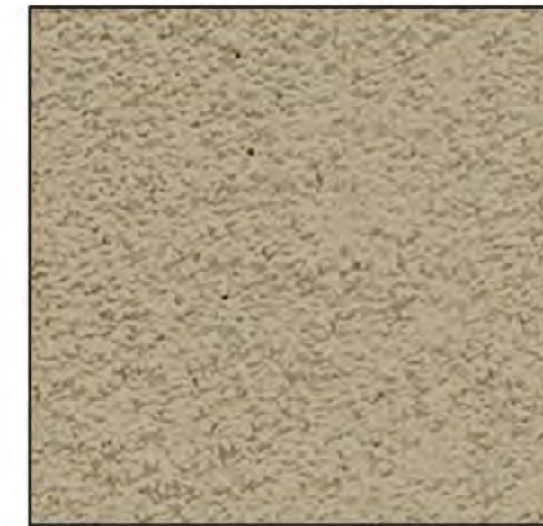
1 EXTERIOR PLASTER WITH SCREEDS OMEGA PRODUCTS INTERNATIONAL SAND FINISH (OR APPROVED EQUAL)
