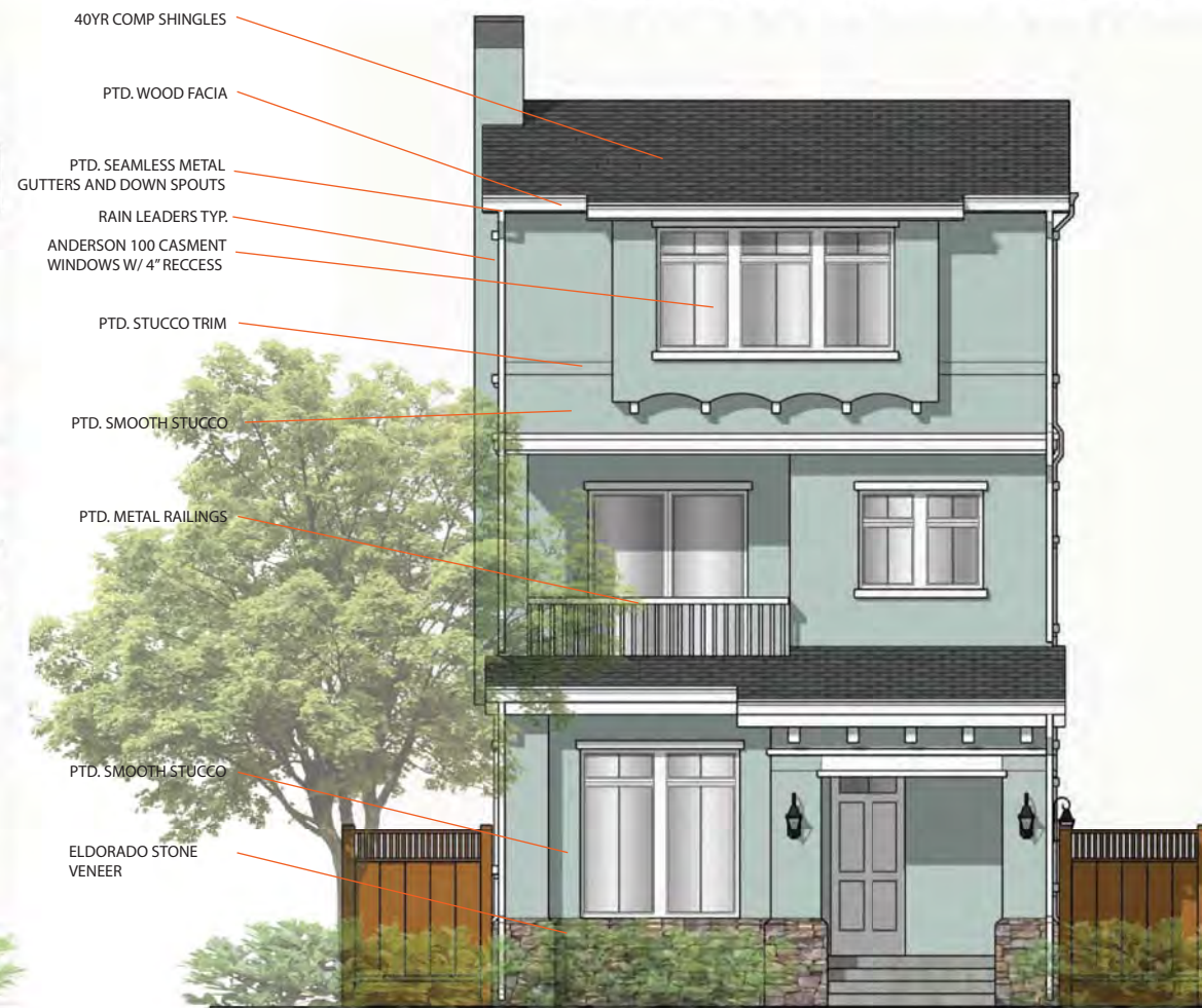
ELEVATION "C" SCALE : 1/4" = 1'-0"
