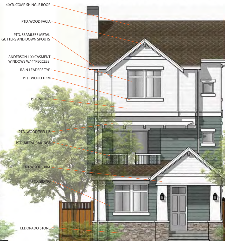
ELEVATION "A" SCALE : 1/4" = 1'-0"
