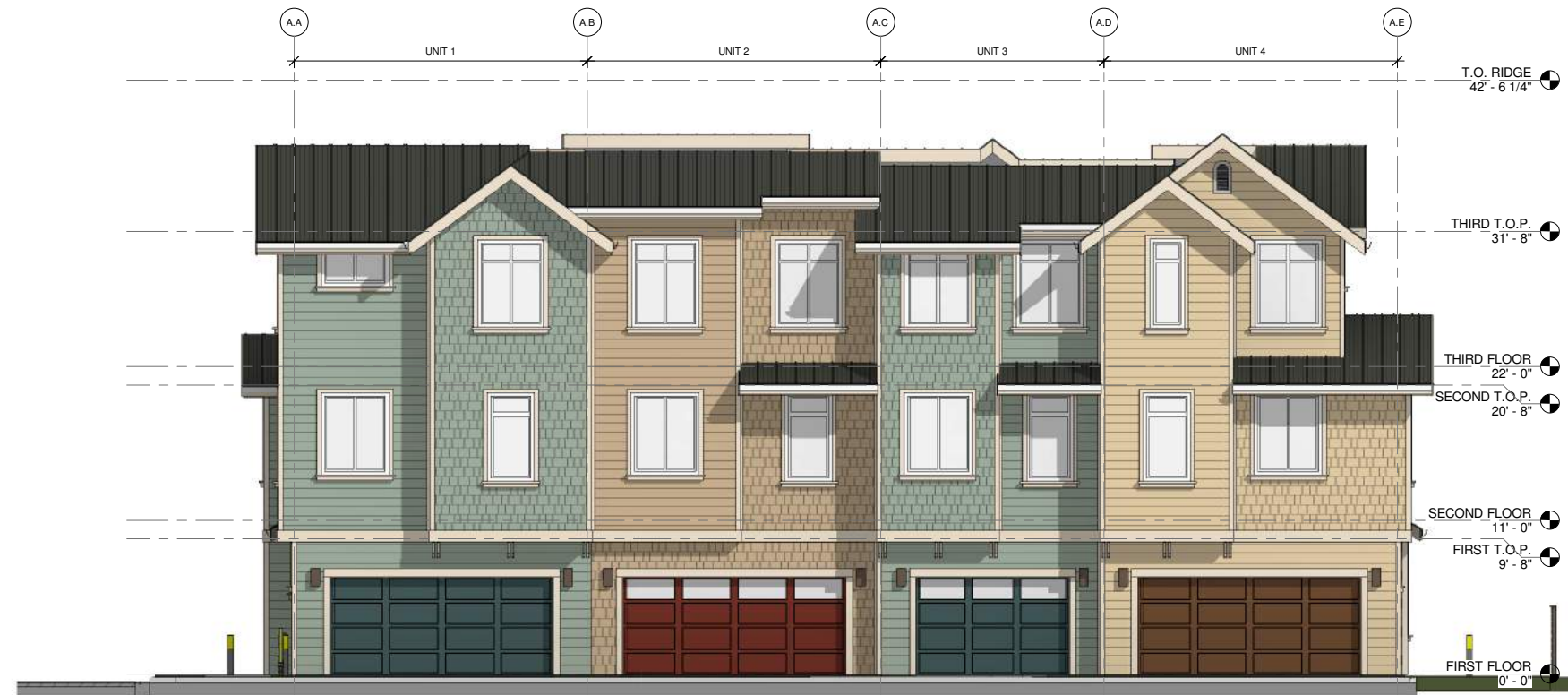
BUILDING A - WEST ELEVATION 3/16" = 1'-0" 2
