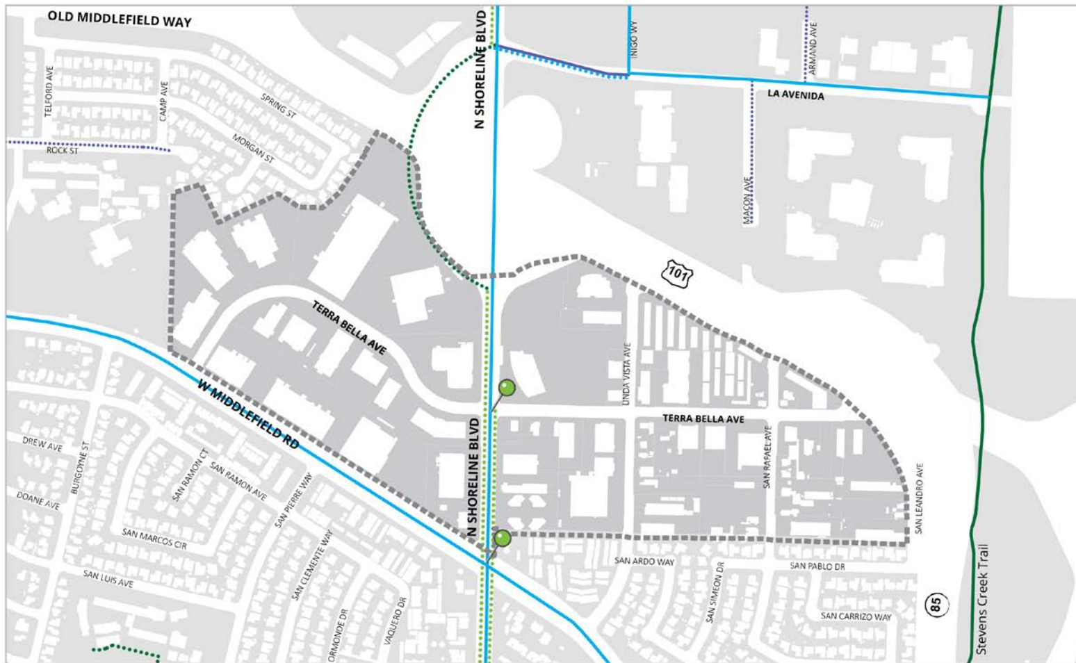
Figure A-9. Existing and Proposed Bicycle Infrastructure
