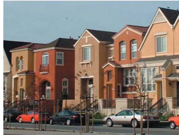
The massing of rowhouses should break the main façade into three or four distinct elements: entry; main facade; a single story element and the roof.
