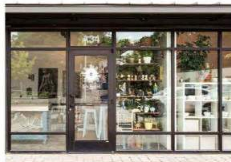
W2 ALUMINUM STOREFRONT - TUBELITE INSIDE FLUSH ANODIZED DARK BRONZE
