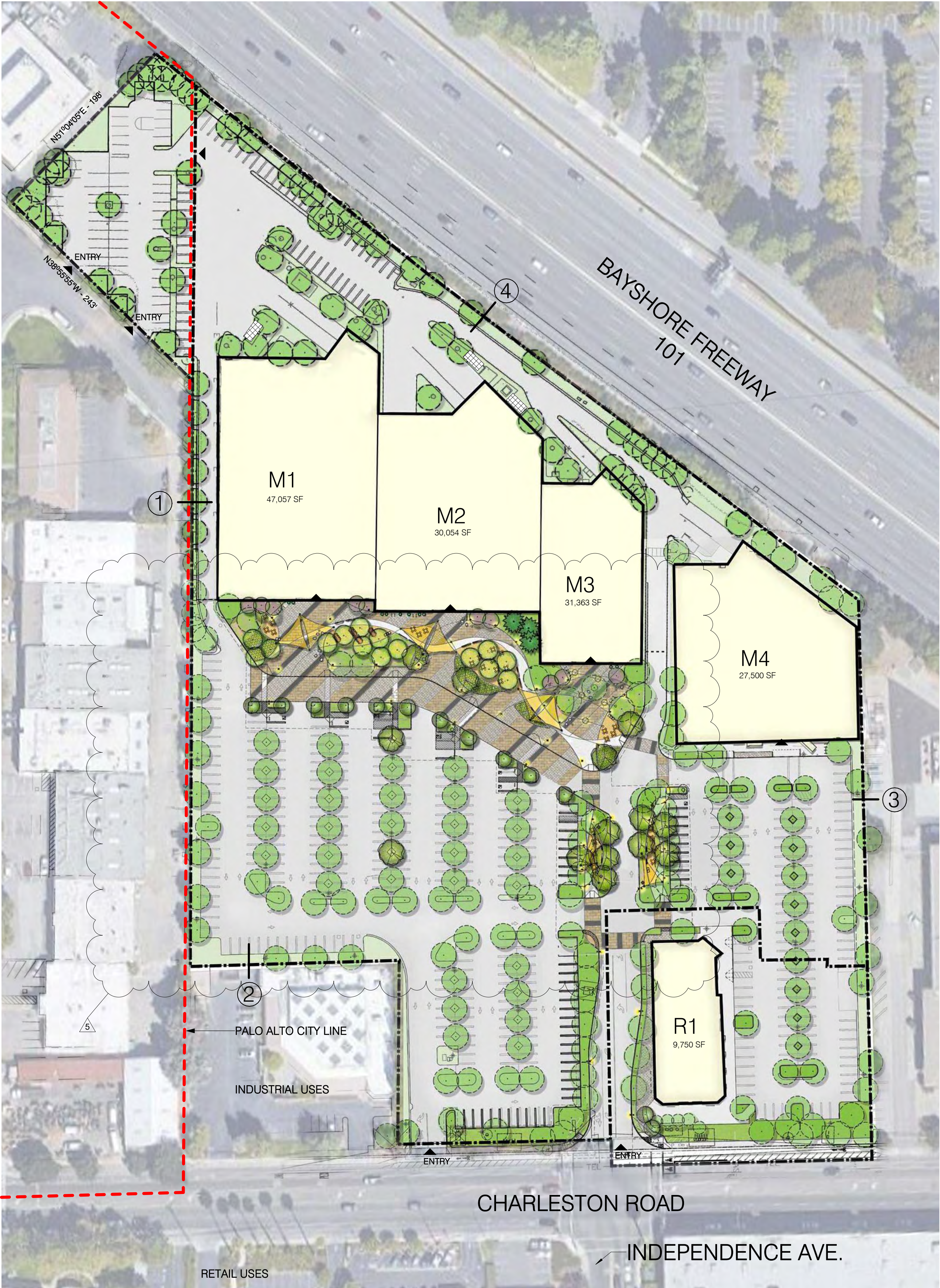
1. WEST PROPERTY LINE - ADJACENT TO BUILDING M1. EXISTING DRIVE ISLE, CURB AND CHAINLINK FENCE. NO PROPOSED MODIFICATION OF GRADES OR PROPERTY BOUDARY WALLS AND/OR FENCING
