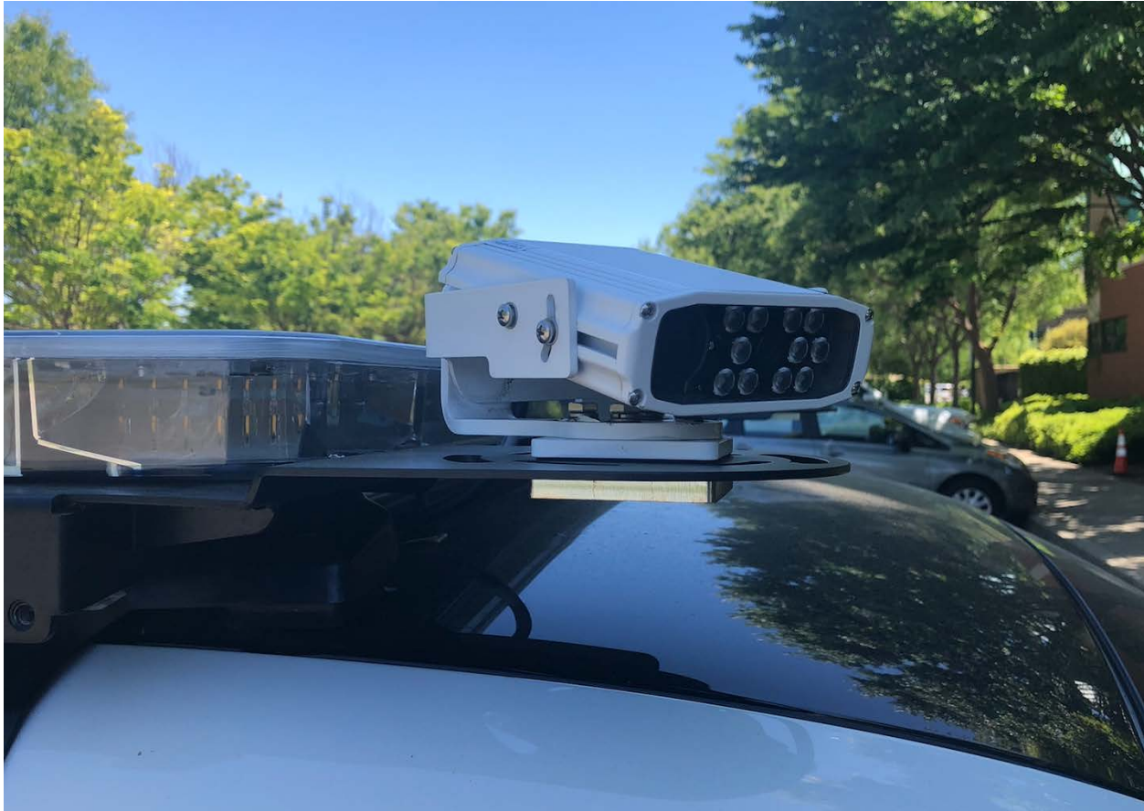
Image 10. Genetec LPR Camera Mounted on City of Davis Enforcement Vehicle
