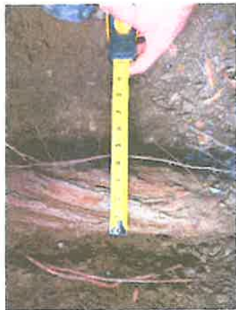
FIG 3: 4" inch root found 24" directly below the concrete footing of the property line retaining wall ( FIG 4 ), which has been uplifted nearly 2' by the roots.
