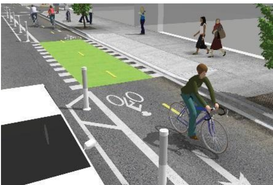
Example of bicycle lane buffer
