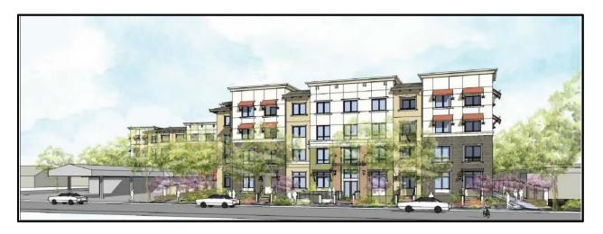
ROEM is proposing a contemporary architectural style, with stone and stucco, a combination of flat and sloped roofs, dark bronze-framed windows, and various accent materials. The design includes a series of complementary paint colors to highlight various projections, floor levels, and articulations on the building exterior. The lobby
