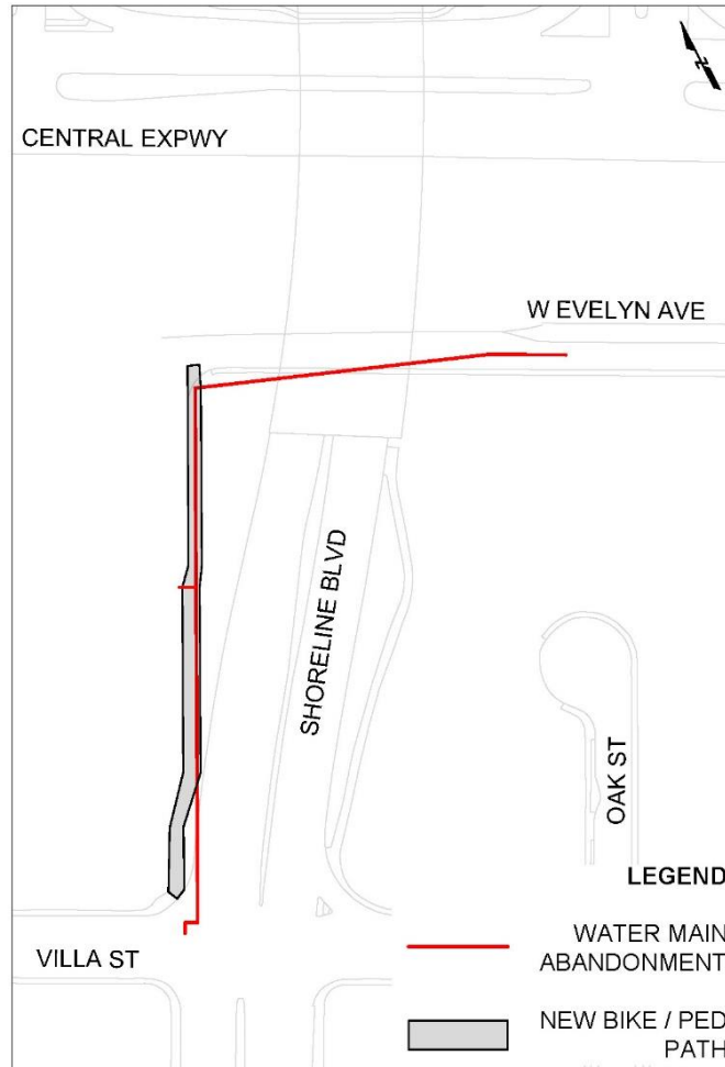
Figure 3: Villa/Shoreline Water Main Abandonment
