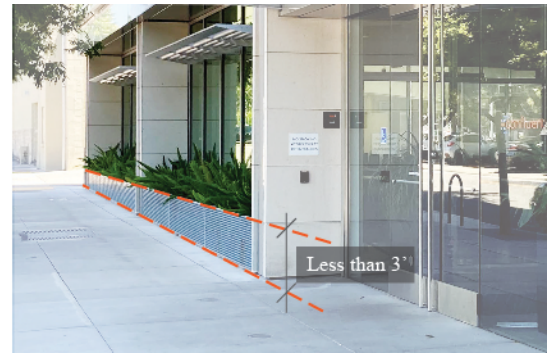
Fig. H.19: Raised planters in setbacks shall not be taller than 3'.
