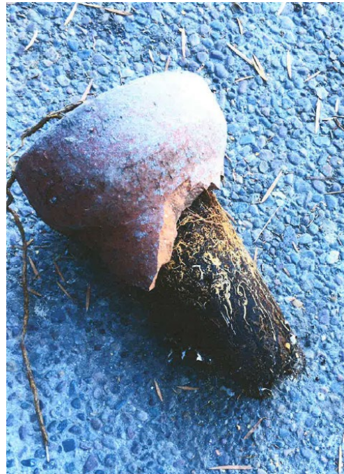
Figure 4: Photo of prior root intrusion of sewer lateral
