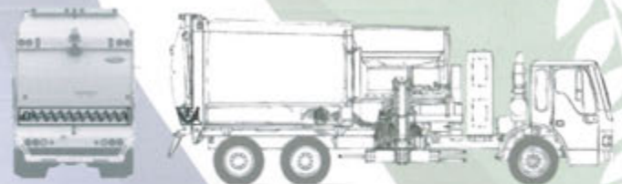
Auger retrofit inserted into tailgate. Allows for dual-use: residential or food waste-only routes.
