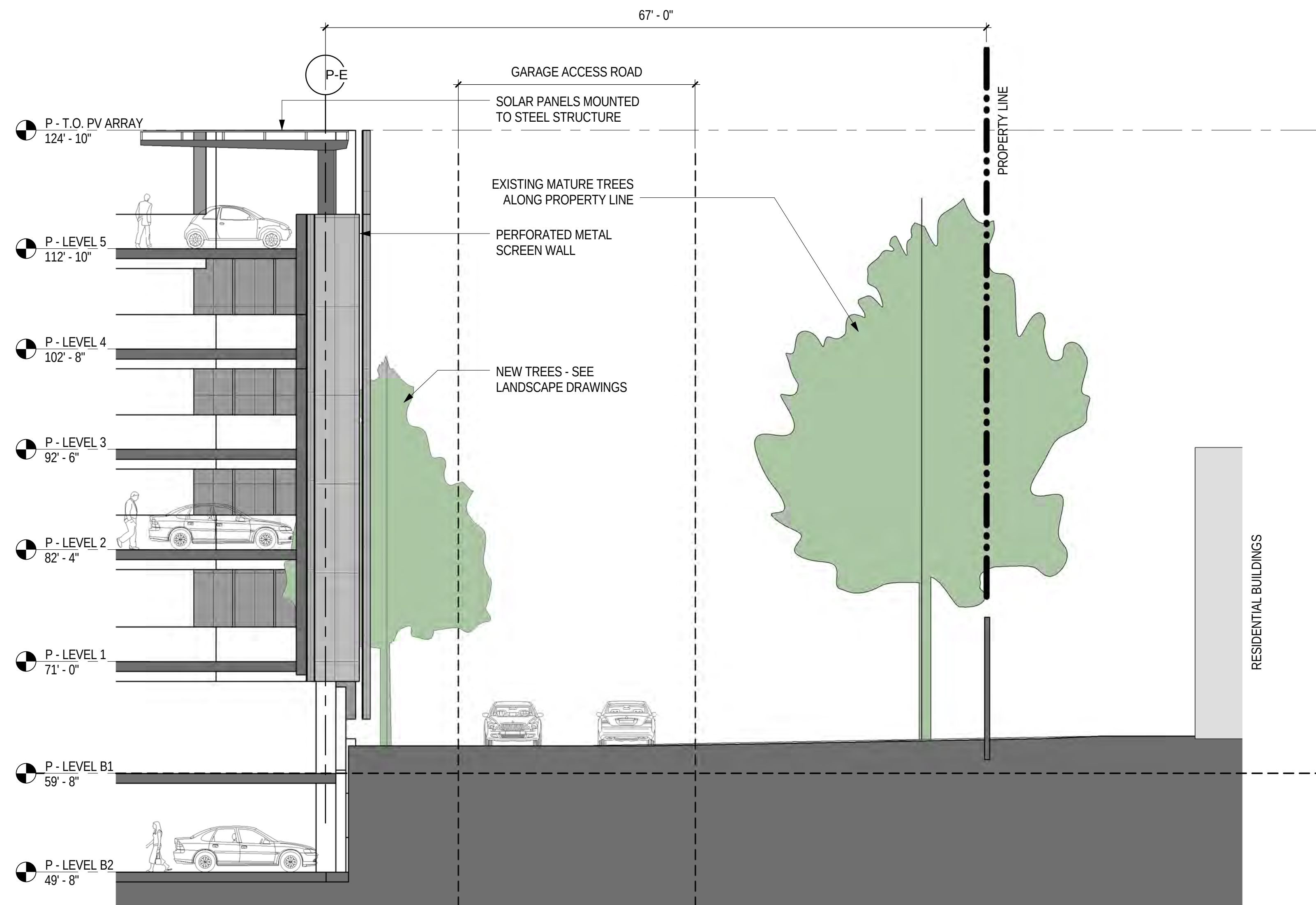
2 BUILDING SECTION - GARAGE 2 ENTRANCE SCALE: 1/8" = 1'-0"
