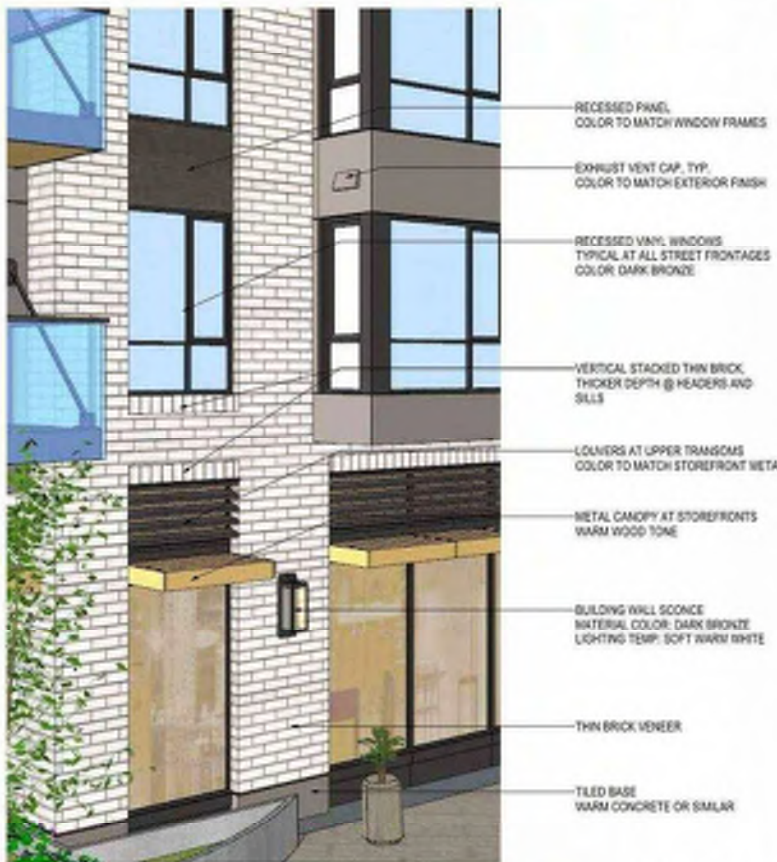
EXTERIOR ELEVATION DETAILS
