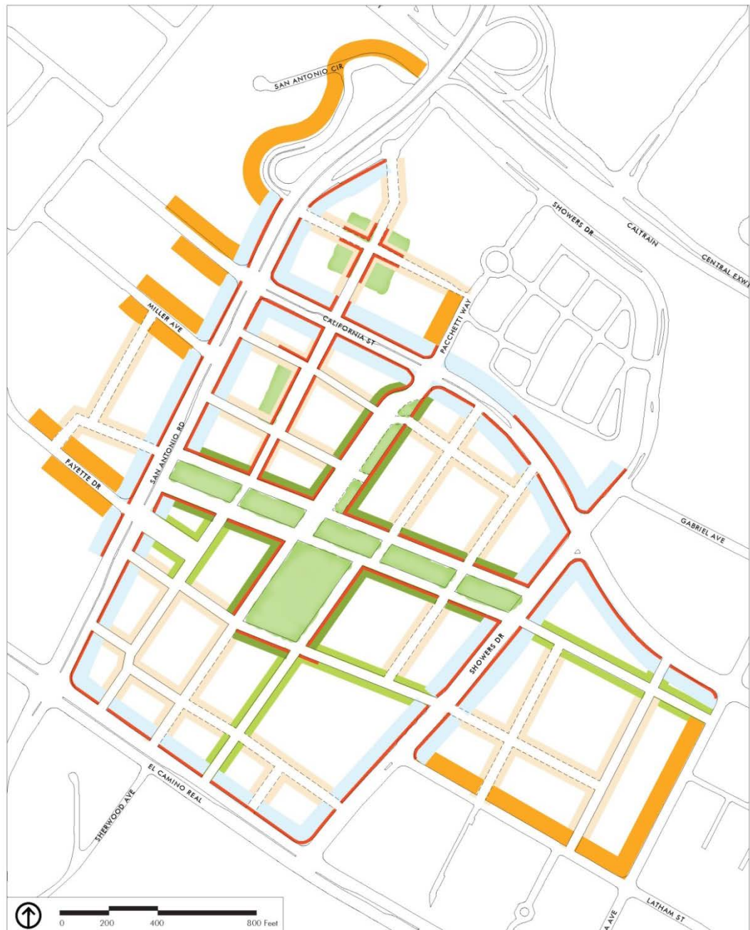
DRAFT Street Types and Active Frontage Space Locations FIGURE 3-2 Major Public Streets Flexible Connections Neighborhood Streets Required Active Frontage Space Greenways Open Space San Antonio Center Internal Streets Precise Plan Area
