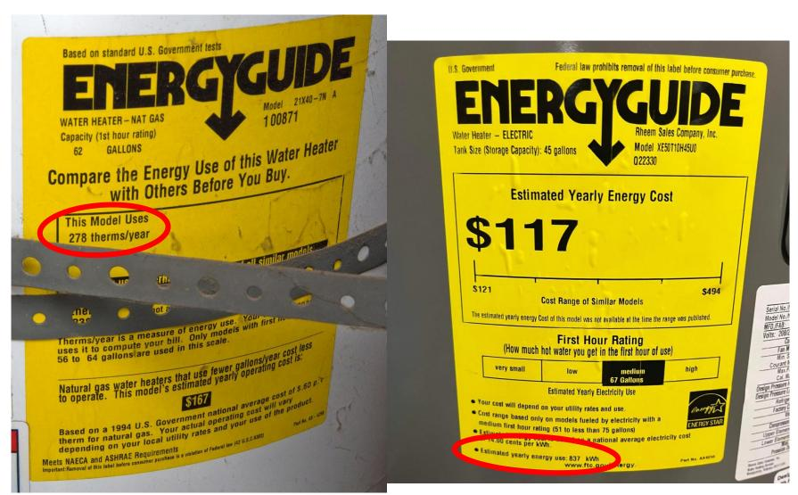
(If  $\sim$ 50% is wasted, 140 therms are used.) (If COP =  $\sim$ 5, 140 therms are moved.)
