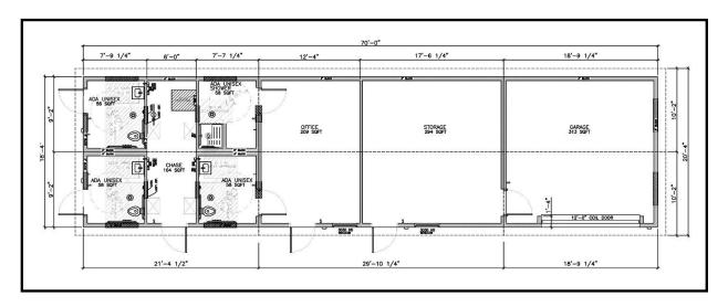
Figure 4: Maintenance Building Floor Plan
