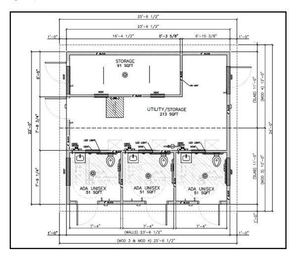
Figure 3: Tennis Building Floor Plan
