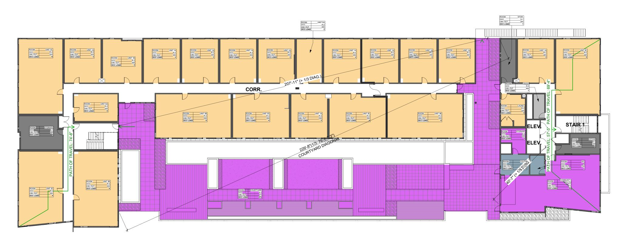
1 3RD FLOOR EXITING DIAGRAM SCALE: 1/16" = 1'-0"
