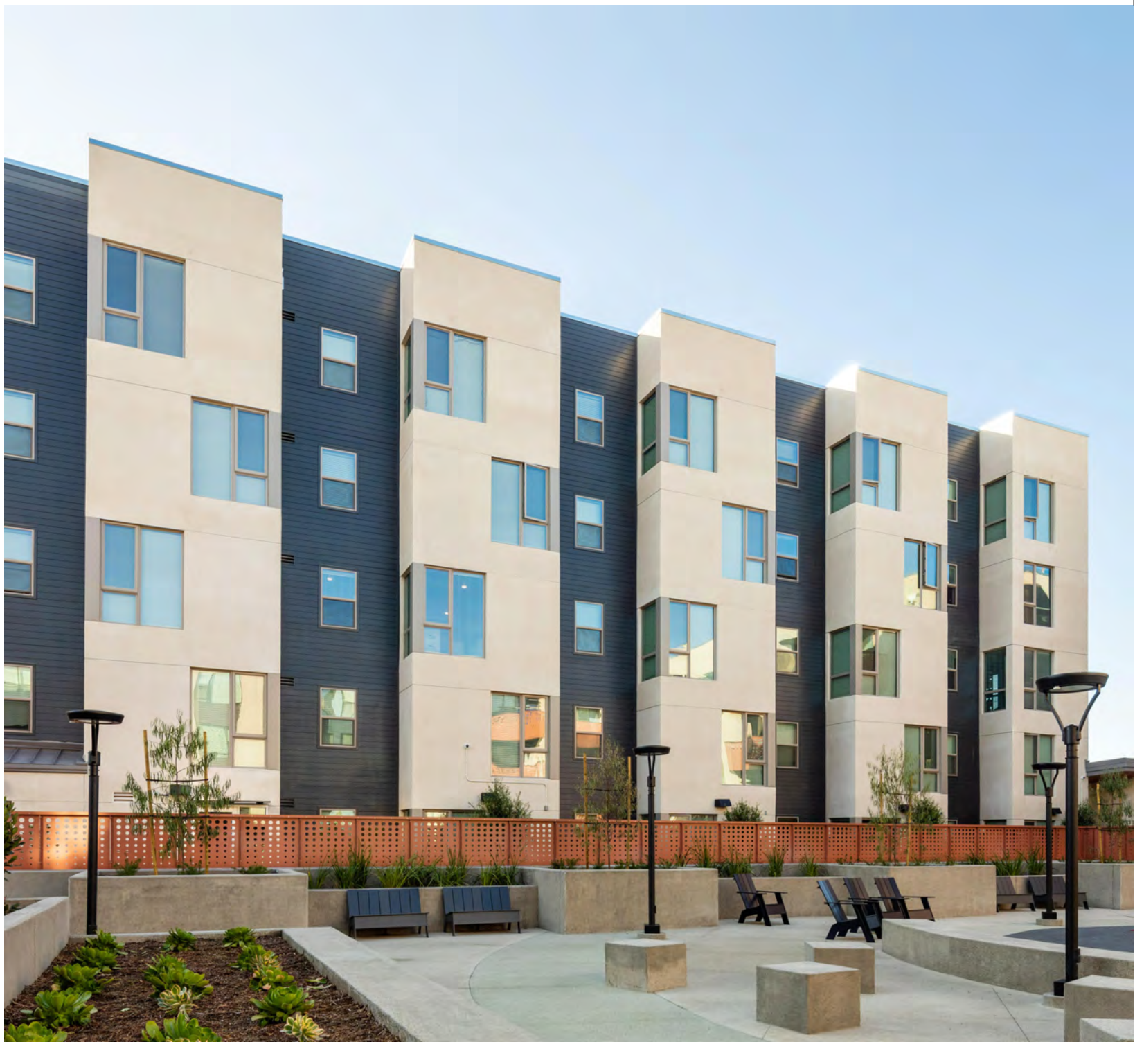
② Plaster Wall with Jogged Parapets, Medium Sand Finish Stucco, Gray Lap Siding, Staggered Windows (Similar to South Elevation)
