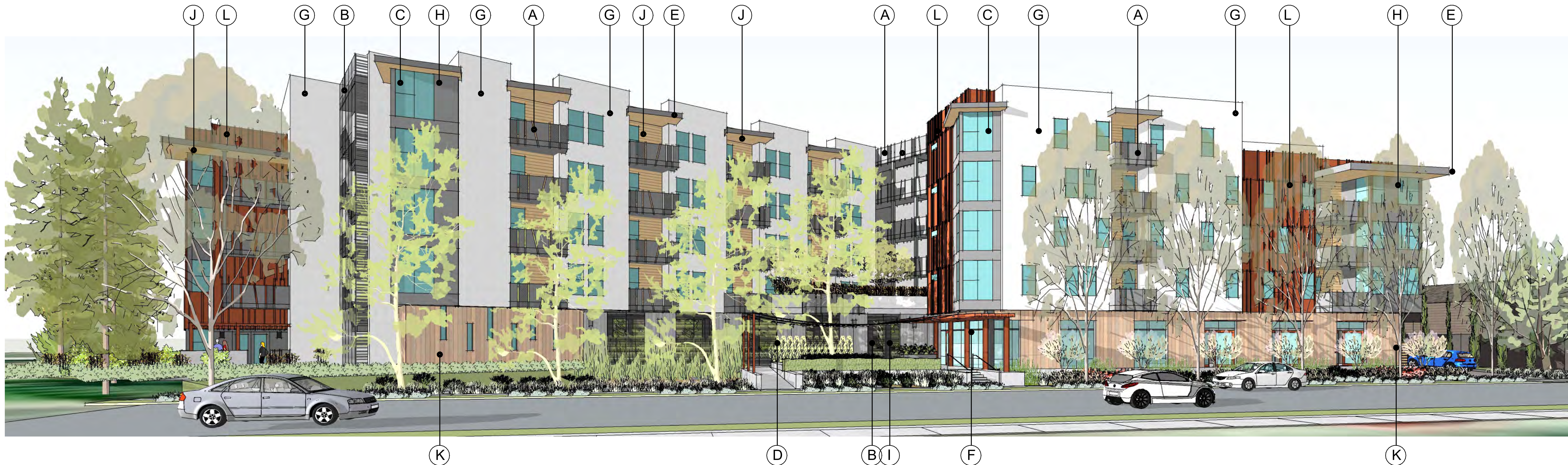
J Horz. Fiber Cement Lap Siding Painted similar to SW 6362 'Tigereye' Basis of Design: HardiePlank Smooth Finish
