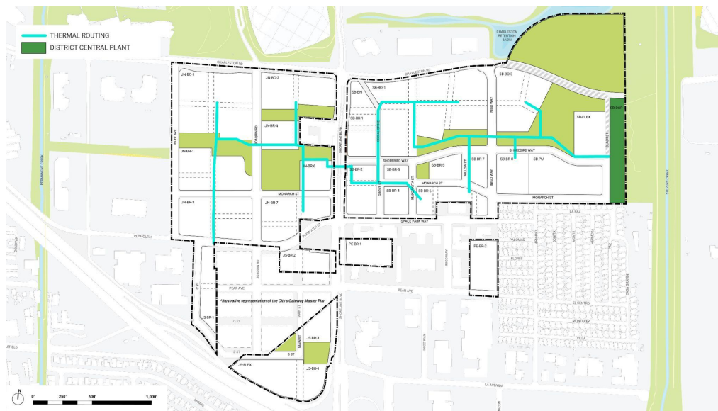
Figure 3.2. CONCEPTUAL THERMAL ENERGY LAYOUT. ILLUSTRATIVE DIAGRAM SUBJECT TO CHANGE.
