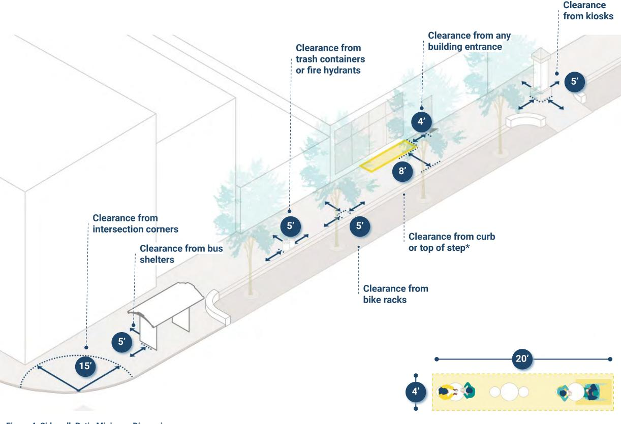
**Figure 4: Sidewalk Patio Minimum Dimensions**
