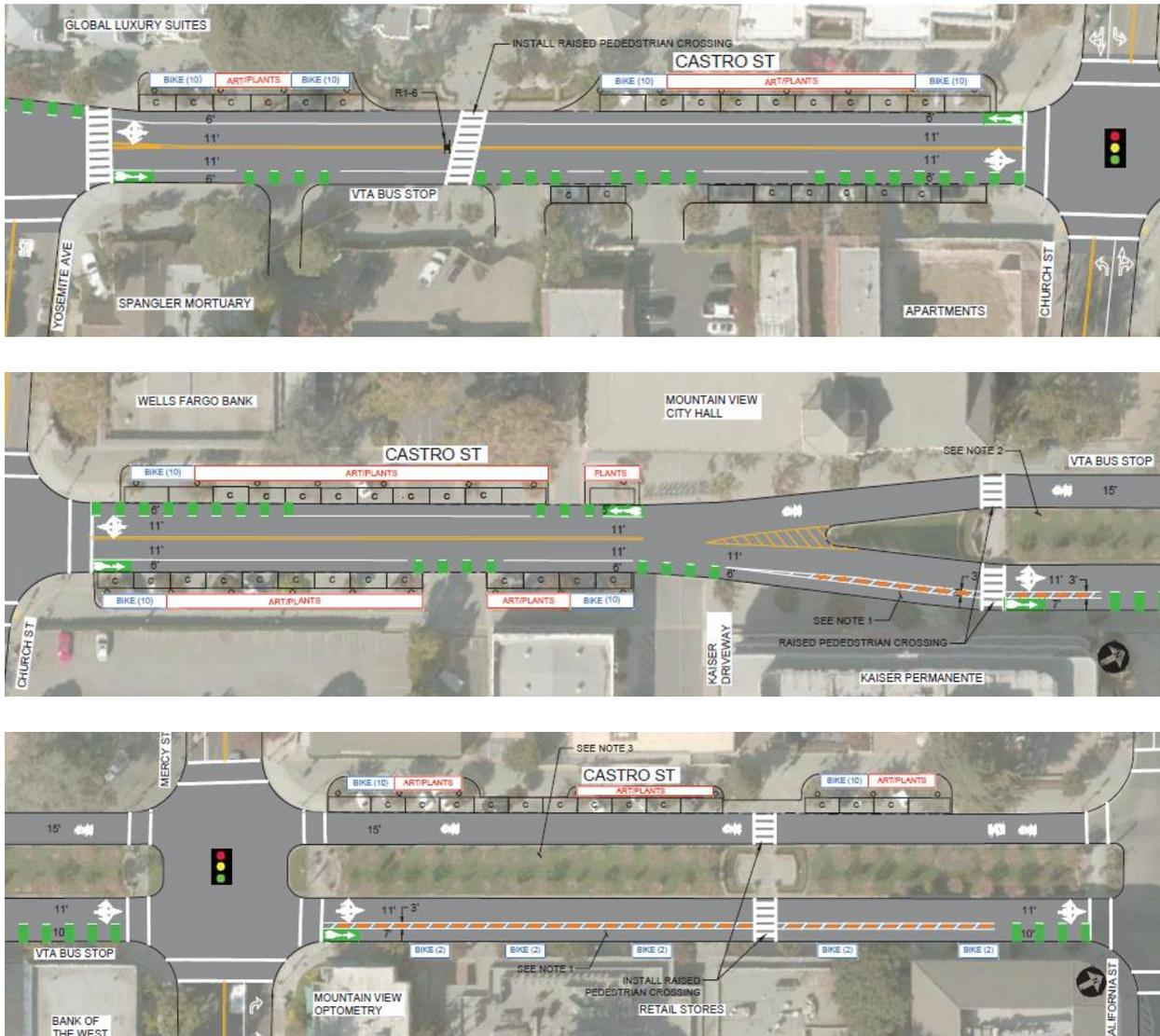
**Figure 6: Short-/Medium-Term Alternative 4—Yosemite Avenue to California Street, More Bike Lanes and Parallel Parking; Remove the 8-Phase Signal at Church Street**
