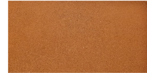
3 GFRC - CLAY COLOR WITH TEXTURED FINISH
