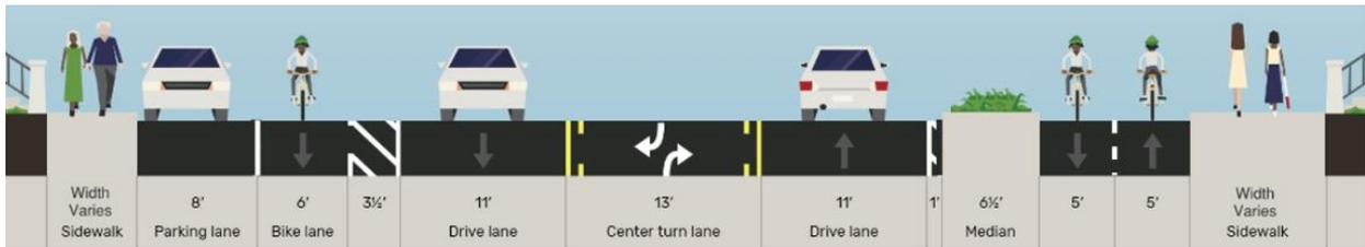
Figure 3: Typical Cross Section of Segment 1
